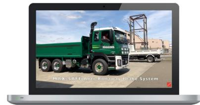
Developed by an Australian company, the **MAX-SAFE Anti-Rollaway Brake System™** provides an active safety solution in the event that the park brake is not fully applied before leaving the vehicle. It provides protection for the driver, occupants, bystanders and workers – while also preventing damage to the vehicle and surrounding property. In Australia, it has been used by thousands of waste management vehicles for a number of years.
